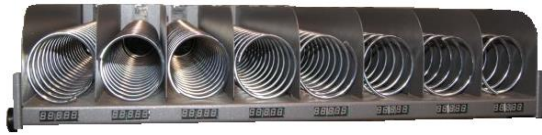
Fig.10 The drawer configured for 8 springs
